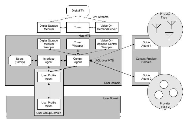
Figure 1: Reference Model for the AVEB Application
